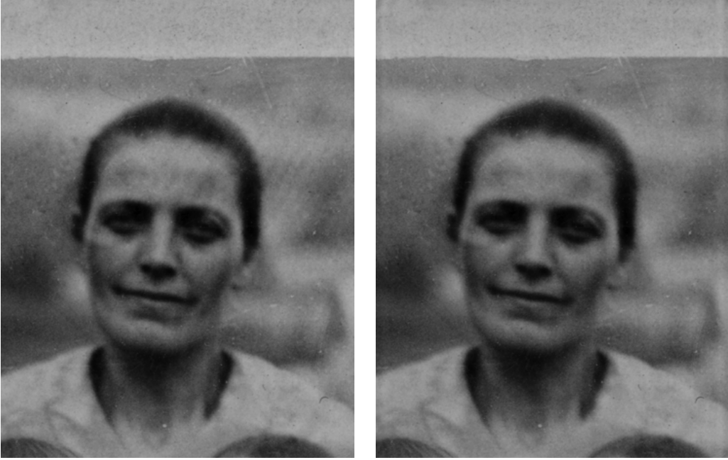
Figure 6: Image with periodic artefact, presumably a finger print. Left: before Right: after notch filtering.
